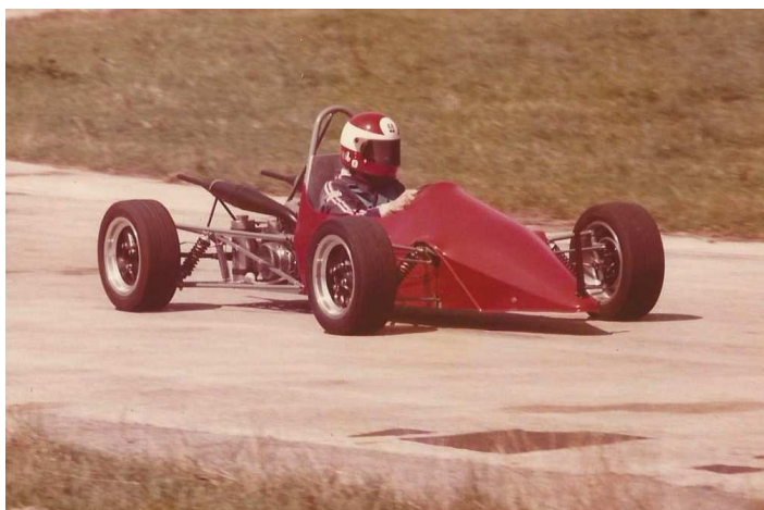
The original car with Suzuki T500 power and number 1A with hybrid Yamaha Tz/Lc500 engine
